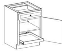
Base Single Door w/Full Width Tray (B_●FWT) Available sizes: Width: 12, 15, 18, 21, 24 Depth: 24 Height: 34½
